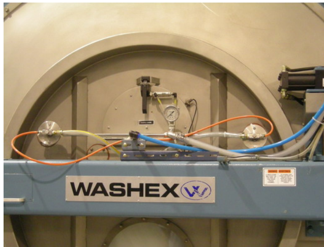
Figure 5. Tandem air atomizing mist spray nozzle configuration on end-of-line LLIN treatment machine.
