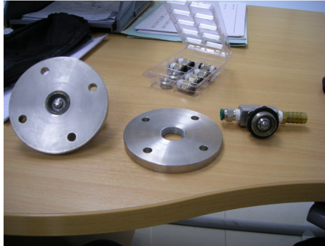
Figure 4. Spraying Systems Company internal mix air atomizing spray nozzles with thru-wall mounting device.
